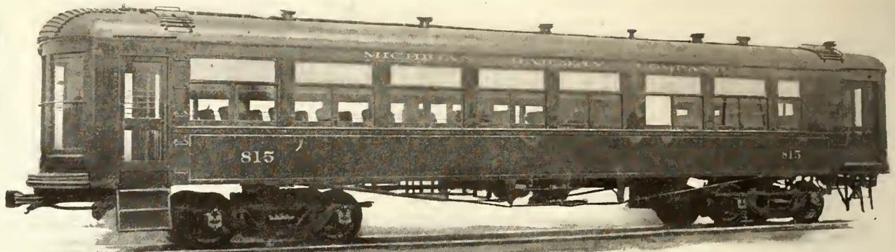
Latest Type Steel Motor Coach Built for the Michigan Railway Company
