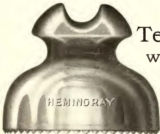
No. 72—Voltages—Test—Dry 64000. Wet 31400. Line 10000.
