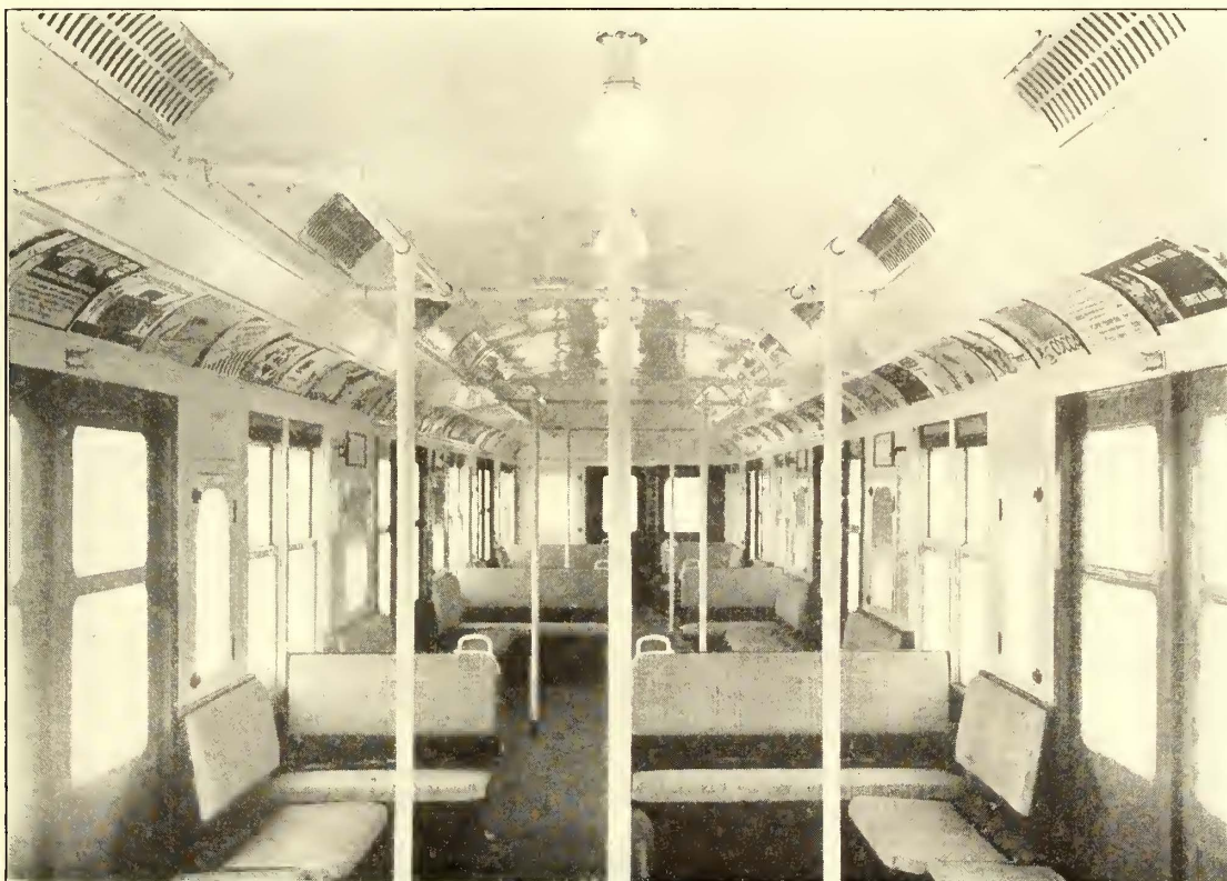
Showing Ellcon Aero Metal Fittings on New York Municipal Railway Car.
