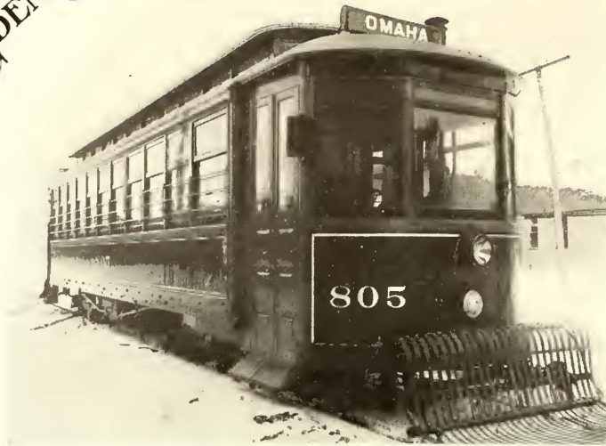
Golden Glow replaced 4 ampere arc and incandescent headlights at Omaha after thorough competitive test.
