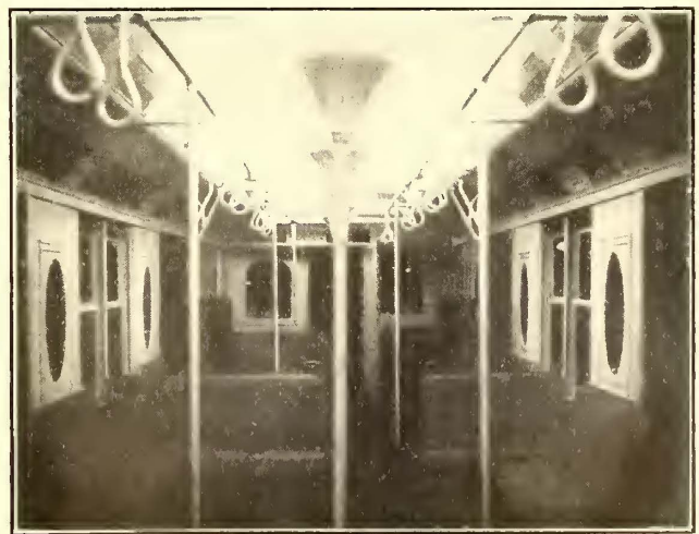
NEW YORK MUNICIPAL CAR—FIG. 18—INDIRECT LIGHTING FROM UNITS ON GRAB RAILS
