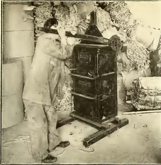
THIRD AVENUE TRANSFER PRINTING—USE OF BALING MACHINE TO TAKE CARE OF TRANSFER TRIMMINGS
