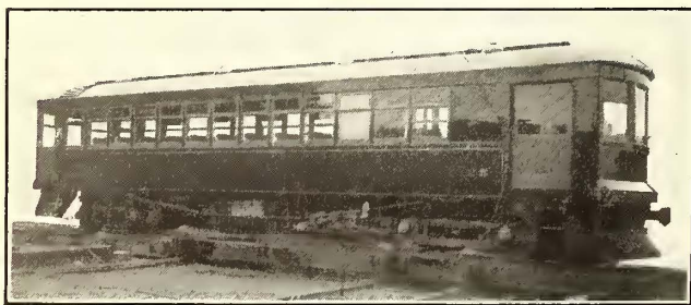
COMBINATION PASSENGER AND BAGGAGE CAR FOR THE KANSAS-OKLAHOMA TRACTION COMPANY
