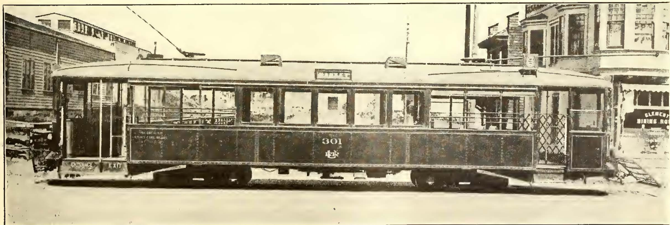
SAN FRANCISCO CAR—SIDE VIEW, SHOWING ARRANGEMENT WITH OPEN SECTIONS AT ENDS OF CAR
