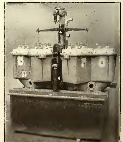
NORFOLK &amp; WESTERN ELECTRIFICATION—PHASE CONVERTER AND LIQUID RHEOSTAT
