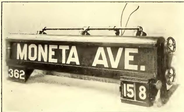
LOS ANGELES CAR SIGN WITH CAR NUMBER PAINTED DIRECTLY ON THE GLASS AND WITH SEPARATE MECHANISM FOR DISPLAYING RUN NUMBER
