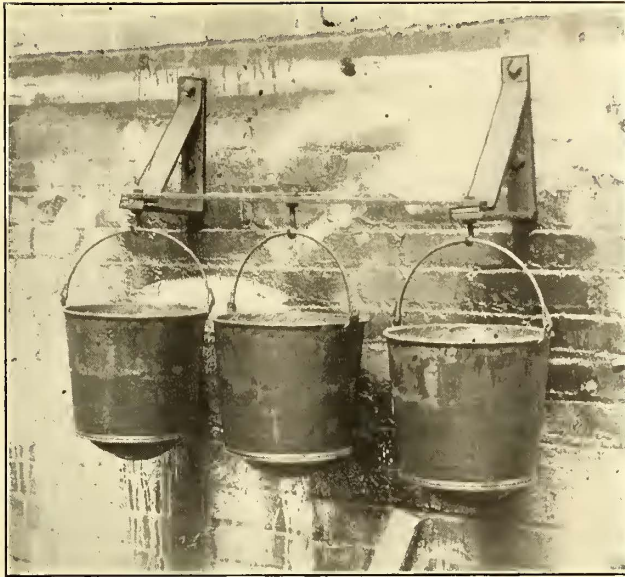
HAMPTON SHOPS—THE SAFE AND CLEAN WAY OF SUSPENDING FIRE PAILS
