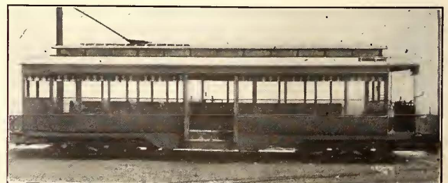
RECONSTRUCTED OPEN CARS—REMODELED CAR WITH STEEL SHEATHING
