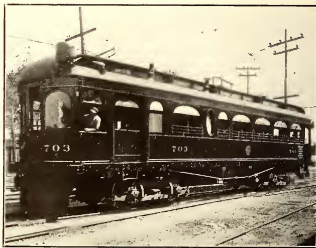
VIEW OF DES MOINES INTERURBAN CAR, SHOWING AIR-OPERATED LOCOMOTIVE BELL
