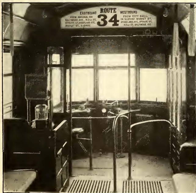
ROUTE SIGNS—PHILADELPHIA SYSTEM—THE VIEW AT THE LEFT SHOWS AN INTERIOR SIGN; THE VIEW AT THE RIGHT SHOWS ROUTE NUMBER AND LINE ON SIDE PANEL AND ROUTE NUMBER AND DESTINATION ON FRONT WINDOW
