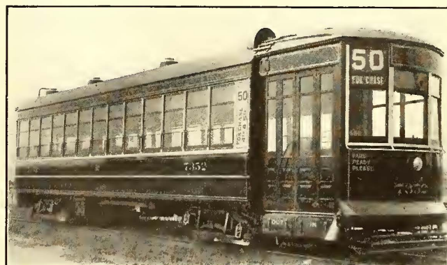
ROUTE SIGNS—PHILADELPHIA SYSTEM—THE VIEW AT THE LEFT SHOWS AN INTERIOR SIGN; THE VIEW AT THE RIGHT SHOWS ROUTE NUMBER AND LINE ON SIDE PANEL AND ROUTE NUMBER AND DESTINATION ON FRONT WINDOW
