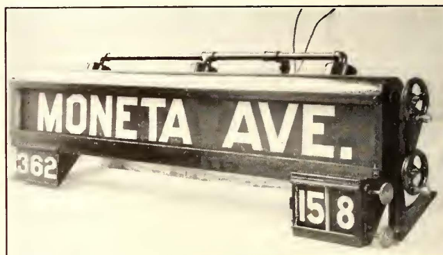
ROUTE SIGNS—LOS ANGELES FRONT-END SIGN WITH ROUTE AND CAR NUMBER
