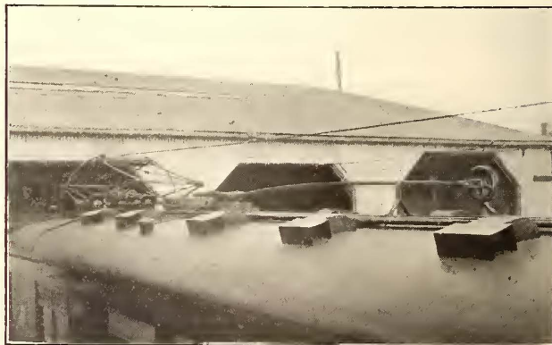
A 10-IN. TROLLEY WHEEL—FIG. 2—PANTOGRAPH UP FOR KEY-ROUTE SECTION AND WHEEL DOWN
