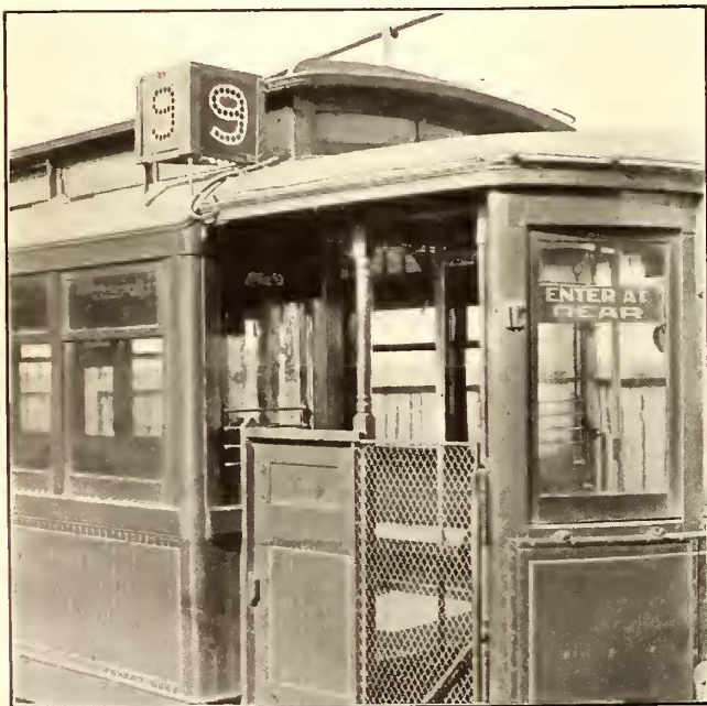
ROUTE SIGNS — PERFORATED METAL SIGN USED BY THE UNITED RAILROADS OF SAN FRANCISCO
