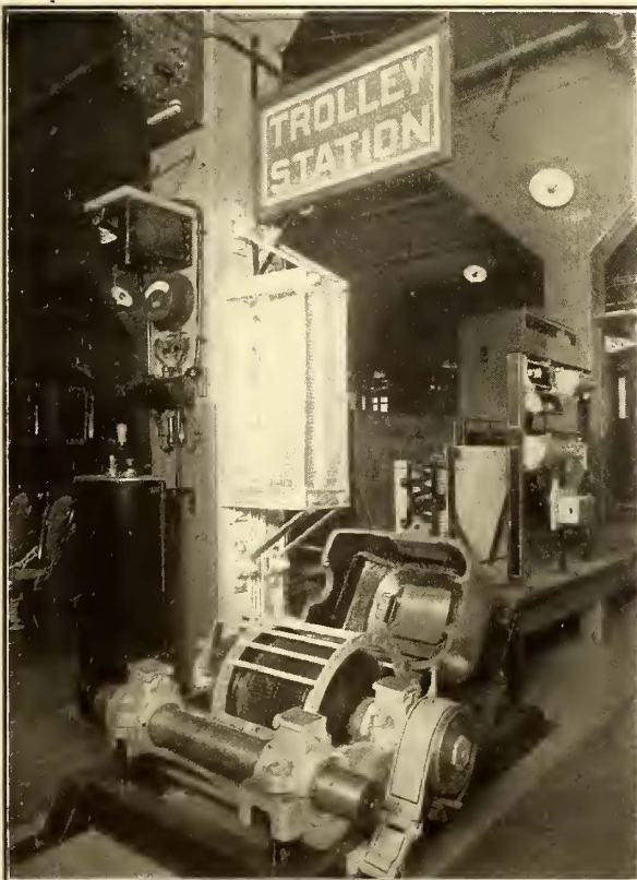
BROOKLYN SURFACE CAR SCHOOL—TEST EQUIPMENT WITH AMMETER AND BANK OF LAMPS TO ILLUSTRATE USE OF MOTOR AS A GENERATOR
