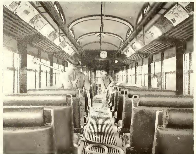
New Vacuum Method of Cleaning
