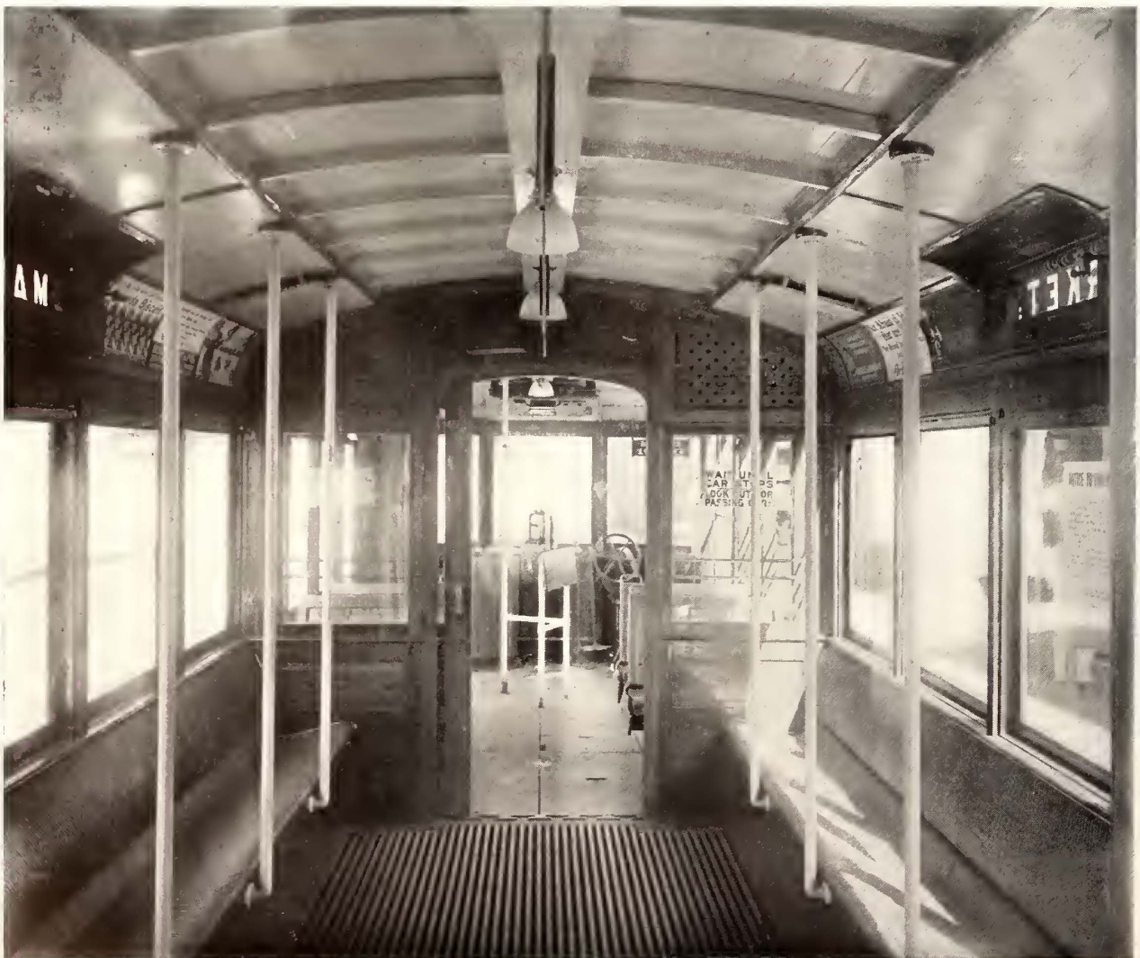
United Railroads Low-Floor Car with Longitudinal Seats in the Center Closed Section and Cross-Seats in the End Sections
