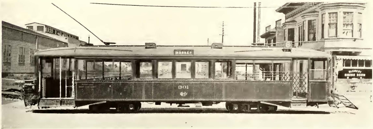
The Latest Car Developed by the United Railroads Is the Low-Floor Type
