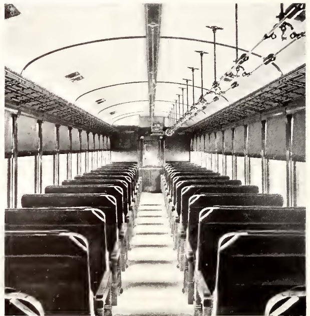
Interior of Latest Pacific Electric Pressed-Steel Car, Showing Seating, Ventilators and Fare Collecting Mechanisms
