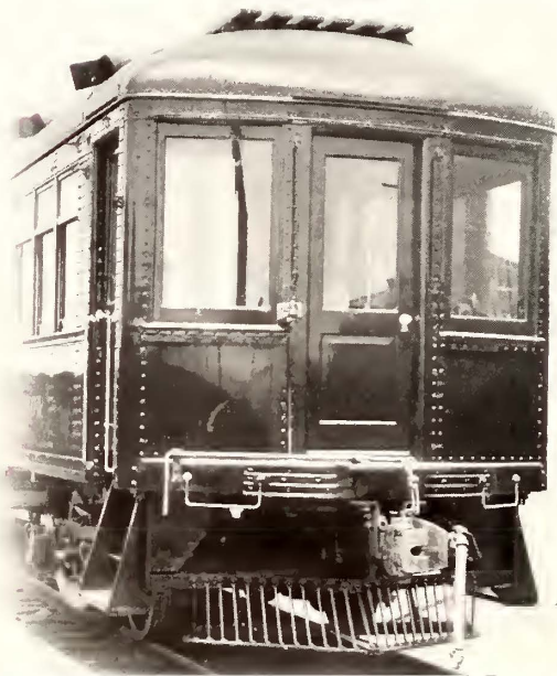
Head-on View of Pacific Electric Pressed-Steel Car, Showing Automatic Air and Electric Coupler, Anti-Climber, Etc.
