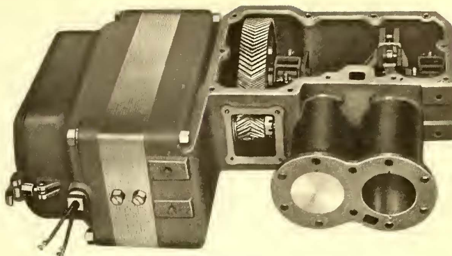
LIGHT-WEIGHT AIR COMPRESSOR—VIEW WITH COVER AND CYLINDER HEAD REMOVED
