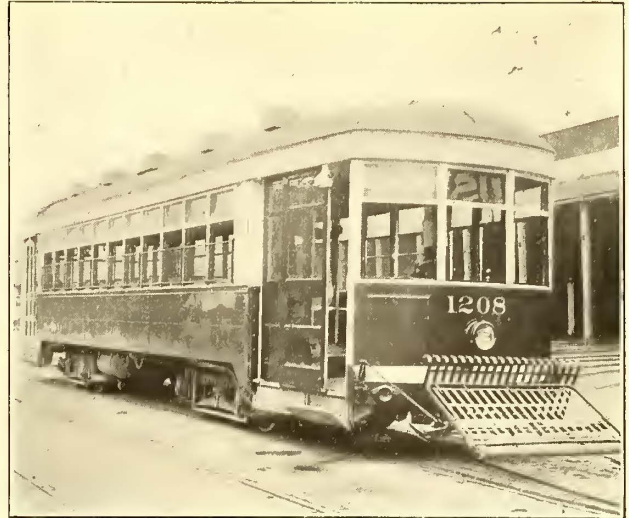
KANSAS CITY CAR—SHOWING STEP LIGHT OVER FRONT DOOR
