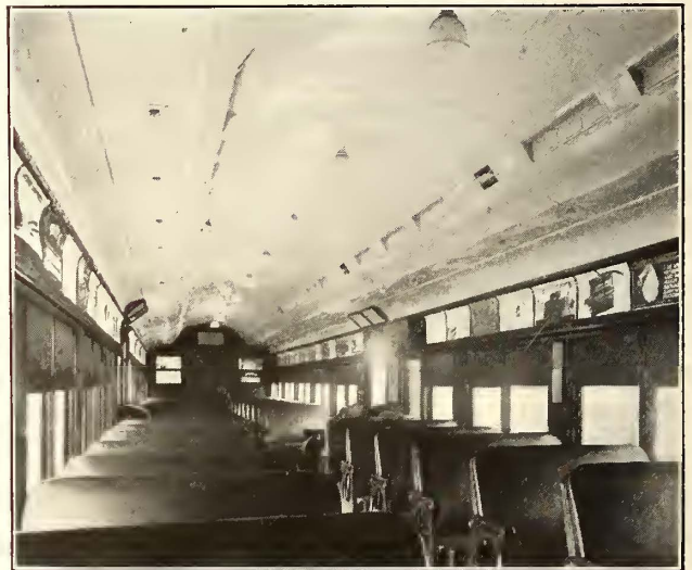
WESTCHESTER LIGHTING—NEW LIGHTING ARRANGEMENT WITH LARGE LAMPS AND REFLECTORS ALONG CENTER LINE OF CAR
