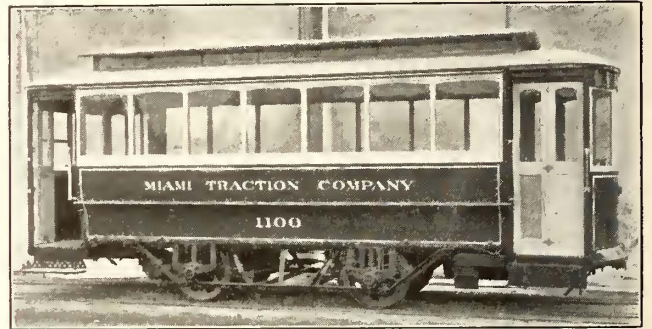
MIAMI CAR—GENERAL VIEW OF STORAGE-BATTERY CAR
