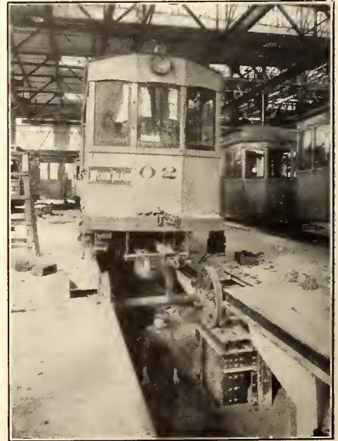
CLEVELAND REPAIR SHOPS—VIEW OF MONORAIL LIFTING CAR CLEAR OF TRUCKS; WHEEL-CHARGING JACK AT RIGHT
