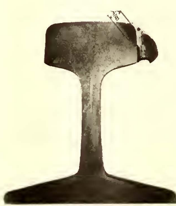
OXY-ACETYLENE WELDING—BOND WELDED TO RAIL HEAD—ETCHING OF RAIL SECTION SHOWING AREA AFFECTED BY WELDING—MICROPHOTOGRAPH OF ETCHED SECTION IN AFFECTED AREA
