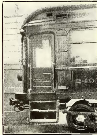
REAR END OF CAR WITH GRAB RAIL; SCALING LADDER AND HANDLES IN SIDE OF CAR
