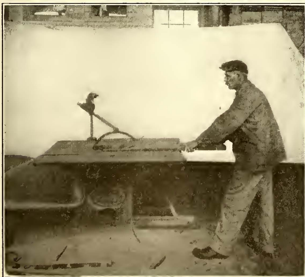
SAFETY ON THE CHICAGO ELEVATED—GUARD ON CIRCULAR SAW
