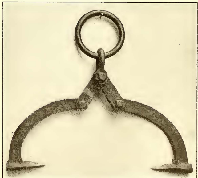
DISTRIBUTING LONG POLES—POLE TONGS
