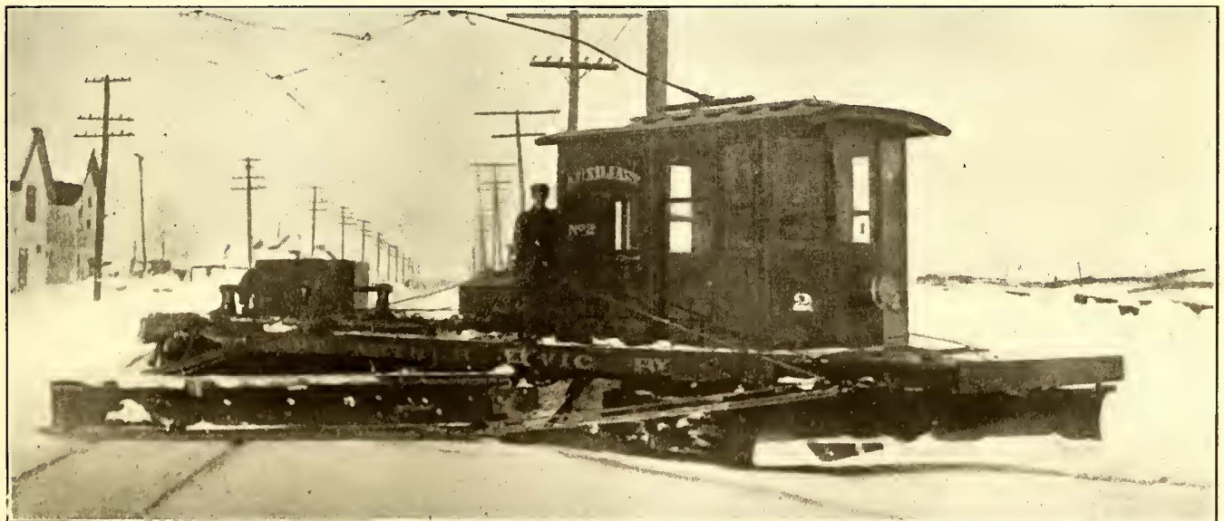
COMBINED WORK CAR, SNOWPLOW AND SWEEPER USED N PORT ARTHUR CIVIC RAILWAY
