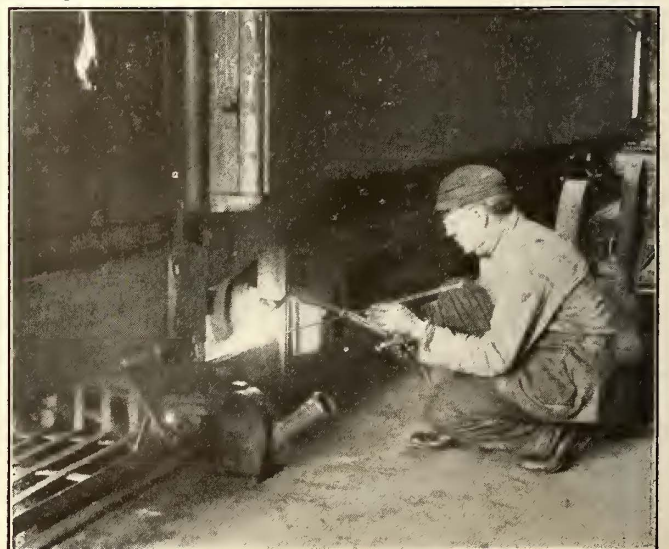
OXY-ACETYLENE REPAIRS—BROKEN TRUCK FRAME WELDED IN PLACE
