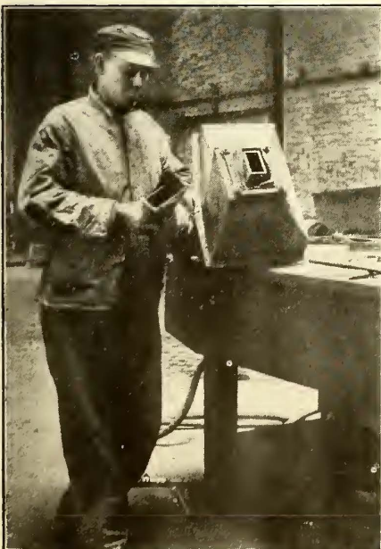
OXY-ACETYLENE REPAIRS—WELDING BROKEN SAND BOX IN FIFTEEN MINUTES
