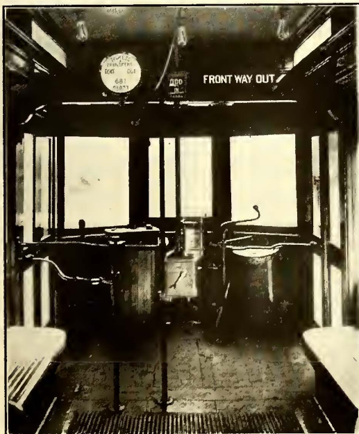
REBUILT CARS—CAB OF SPRINGFIELD CAR LOOKING TOWARD CONDUCTOR'S POSITION AND SHOWING DOOR, STEP-OPERATING HANDLE, FARE BOX AND REGISTERS; INTERIOR OF WORCESTER CAR CONVERTED FROM TWELVE-BENCH OPEN CAR
