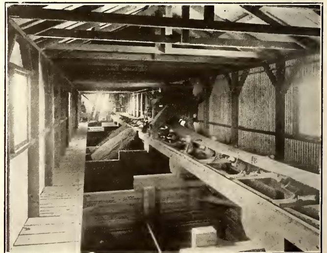
S. F.-O. T. RYS. PAVING PLANT—BELT CONVEYOR WITH TRIPPER OVER STORAGE BINS
