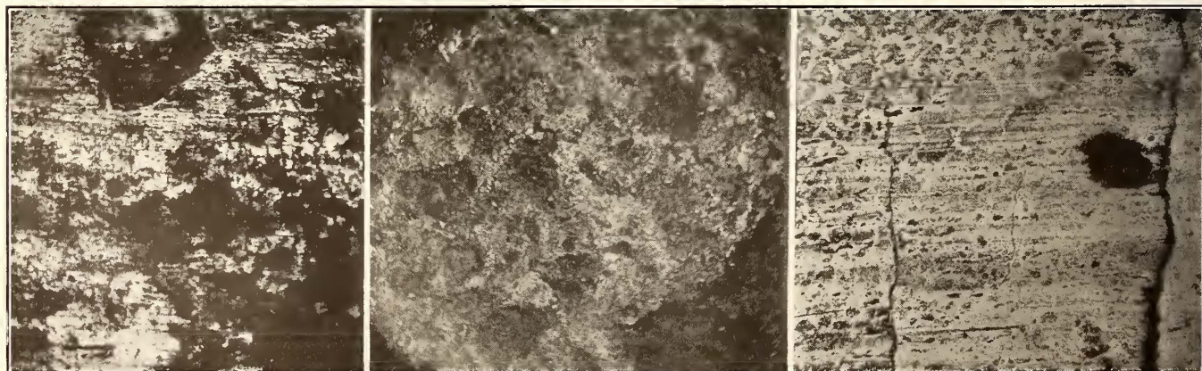
RAIL CORRUGATION—FIGS. 2 AND 3—NATURAL SURFACES OF CREST AND HOLLOW, RESPECTIVELY, OF CORRUGATED RAIL, MAGNIFIED 13\frac{1}{2} DIAMETERS; FIG. 4—SURFACE OF CREST, MAGNIFIED 110 DIAMETERS
