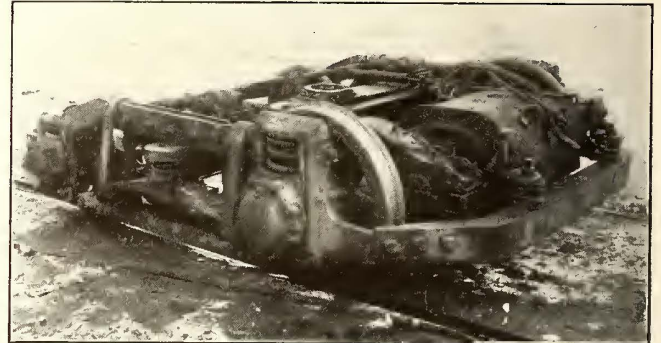
ROCHESTER CAR—VIEWS OF MAXIMUM TRACTION TRUCKS WITH 24-IN. DRIVING WHEELS
