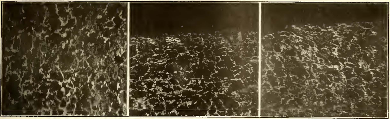
RAIL CORRUGATION—FIG. 5—SURFACE OF HOLLOW, 110 DIAMETERS; FIGS. 6 AND 7—LONGITUDINAL SECTIONS AT CREST AND HOLLOW, 110 DIAMETERS
