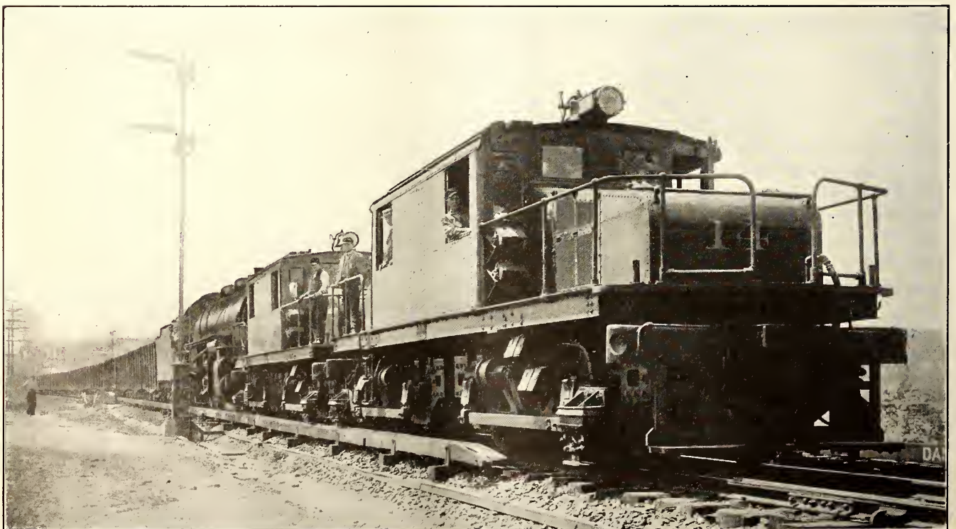
B. & O. ELECTRIFICATION—TWO ELECTRIC LOCOMOTIVES OF 1910 TYPE HAULING FREIGHT TRAIN AND ITS STEAM LOCOMOTIVE
