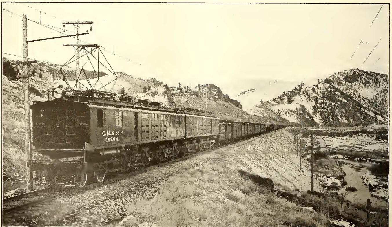
ST. PAUL ELECTRIFICATION—EIGHTY-TWO-CAR FREIGHT TRAIN HAULED BY SINGLE ELECTRIC LOCOMOTIVE
