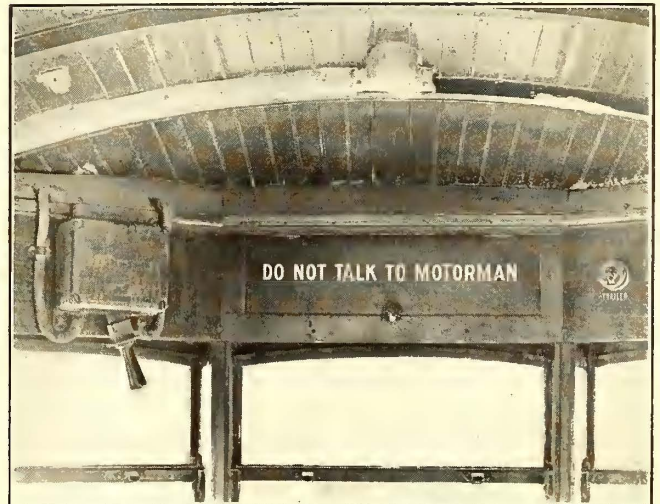
SEALED FUSE CABINET ON MILWAUKEE ELECTRIC RAILWAY CARS
