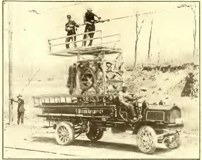
THIRD AVENUE LINE TRUCKS—3-TON TOWER TRUCK IN SERVICE
