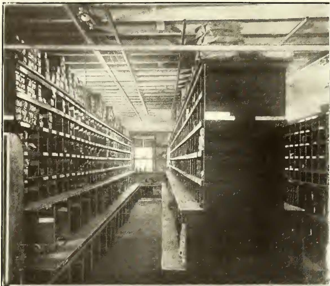
COLUMBUS STOREHOUSE SYSTEM—VIEW SHOWING METHOD OF MARKING ON ENDS OF BINS
