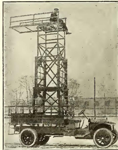
TRENTON THREE-SECTION TOWER TRUCK FOR GENERAL MAINTENANCE WORK
