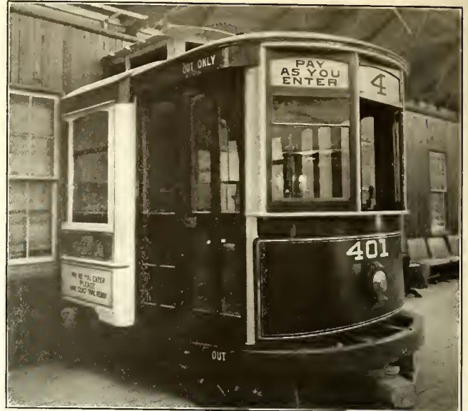
REMODELING BALTIMORE CARS—DUMMY VESTIBULE FROM EXIT SIDE
