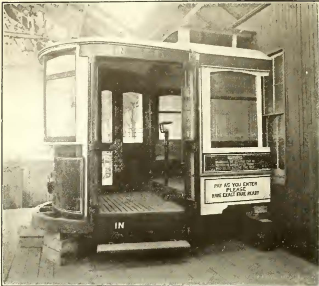
REMODELING BALTIMORE CARS—DUMMY VESTIBULE FROM ENTRANCE SIDE
