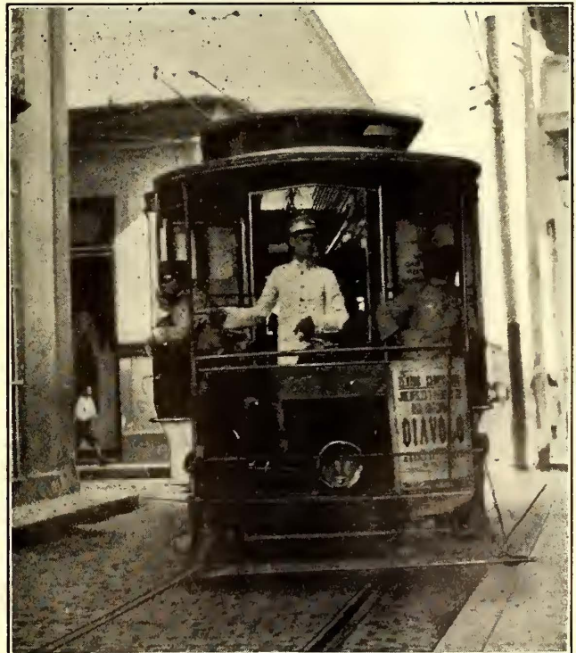
HAVANA—NARROW STREET SHOWING HOW FENDERS PROJECT OVER SIDEWALK WHEN CAR IS ON CURVE
