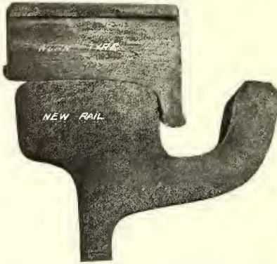
CROSS SECTIONS OF LEEDS 1910 CURVED HEAD RAIL AND WORN TIRE SHOWING INTIMATE CONTACT OF TREADS
