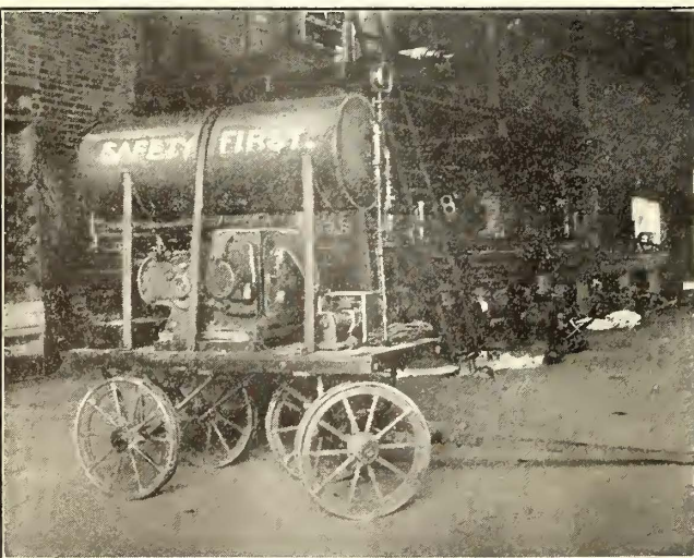
AIR COMPRESSOR MOUNTED ON A TRUCK IN SHOPS OF BENTON HARBOR-ST. JOE RAILWAY
