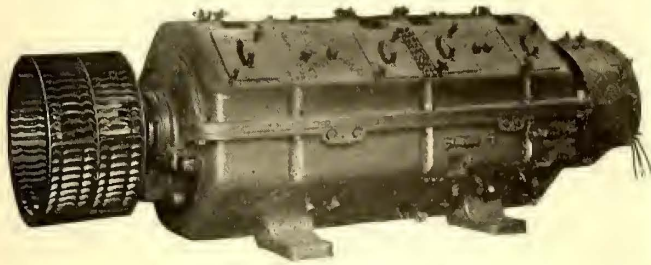
C., M. & ST. P. LOCOMOTIVES—MOTOR-GENERATOR SET WITH FAN HOUSING REMOVED
