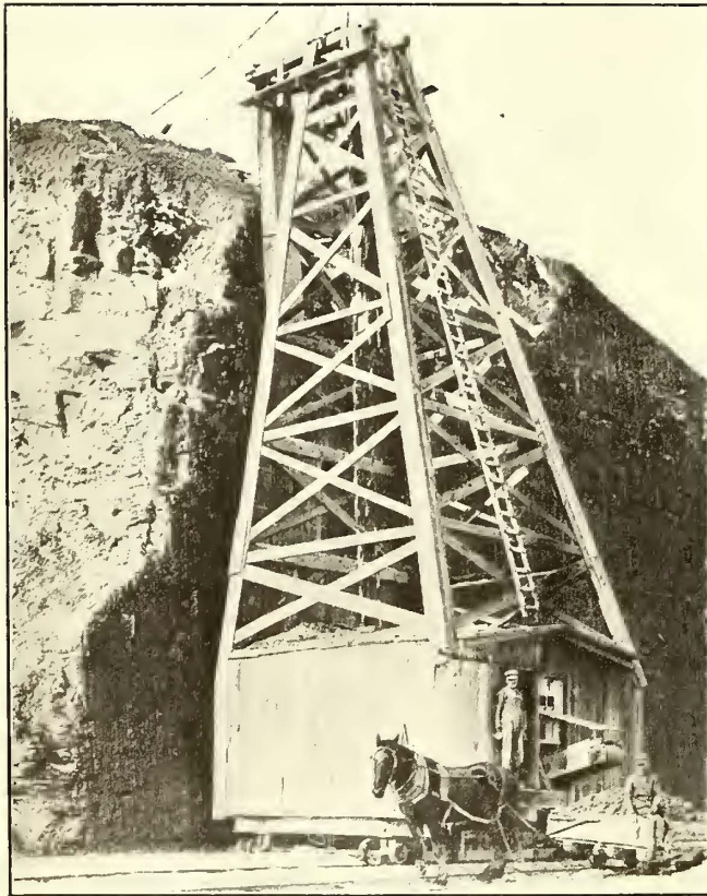
INTERURBAN POWER SALES—EQUIPMENT IN INDIANA SHALE QUARRY OPERATED BY D.-C. MOTOR ON INTERURBAN TROLLEY CIRCUIT
