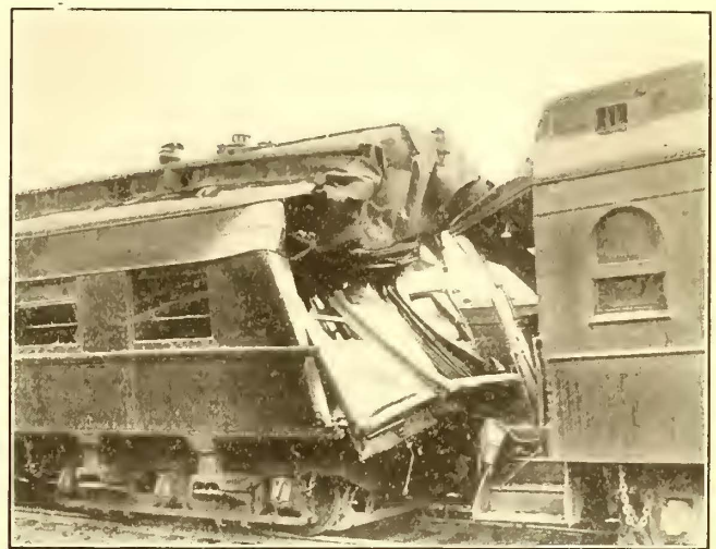
TRUSS-SIDE CARS—EFFECT OF COLLISION ON CAR WITH LIGHT SUPERSTRUCTURE
