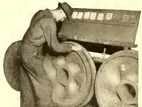
Taping Davis Steel Wheels to insure proper mating in service
