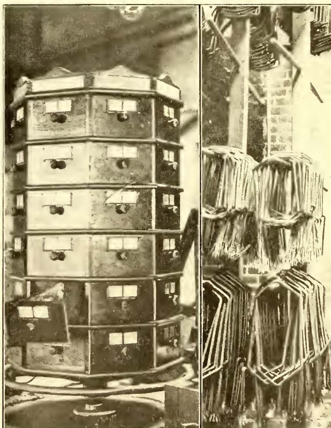
FIG. 2—SCREW CABINET; FIG. 3—ARMATURE COIL STORAGE RACK UNIT. BOTH IN RHODE ISLAND COMPANY'S SHOPS
