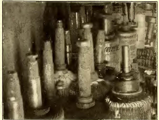
ARMATURE SHAFTS BUILT UP BY ARC WELDING
