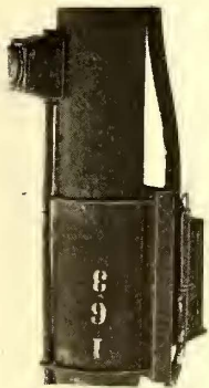
CONDULET ATTACHED TO TROLLEY POLE
