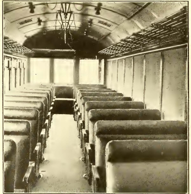
JAMESTOWN CARS—INTERIOR VIEW OF PASSENGER COMPARTMENT, SHOWING FULLY GLAZED MOTORMAN'S COMPARTMENT IN RIGHT-HAND CORNER
