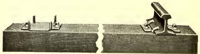
TIE PLATE BEFORE AND AFTER CLAMPING TO RAIL
