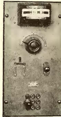
TEMPERATURE INDICATOR SWITCHBOARD
