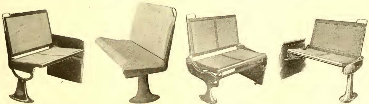
Four Types of Seats Used on Light-Weight Safety Cars. Fig. 1—A 24-lb. Non-Reversible Seat. Fig. 2—Seat with Concave Convex Cushion and Back. Fig. 3—Seat Used Extensively by the Illinois Traction System. Fig. 4—Reversible Seat Used on Birney Cars
