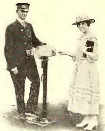
Transfer-Issuing Machine in Operation
