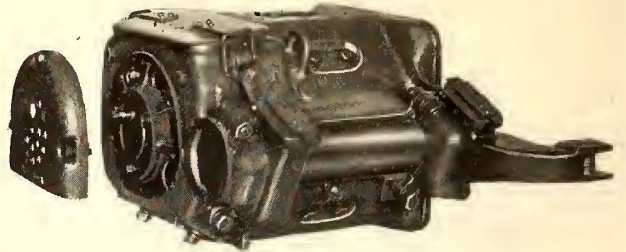
General View of GE-258 Motor for Light-Weight Safety-Car Service—Rating 25 Hp., 600 Volts
