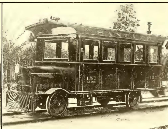
WESTERN GASOLINE CARS—SANTA FÉ CAR MADE UP OF SPECIAL BODY ON AUTOMOBILE CHASSIS
