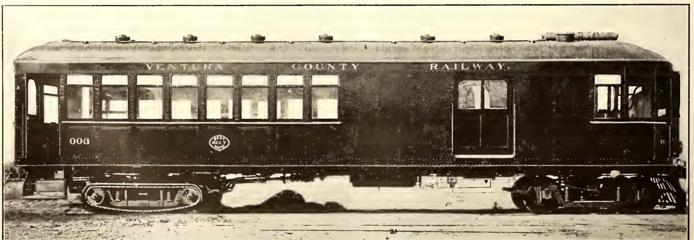
WESTERN GASOLINE CARS—PASSENGER CAR THAT SERVES ALSO AS FREIGHT LOCOMOTIVE AND HANDLES ENTIRE SERVICE ON 21-MILE LINE
