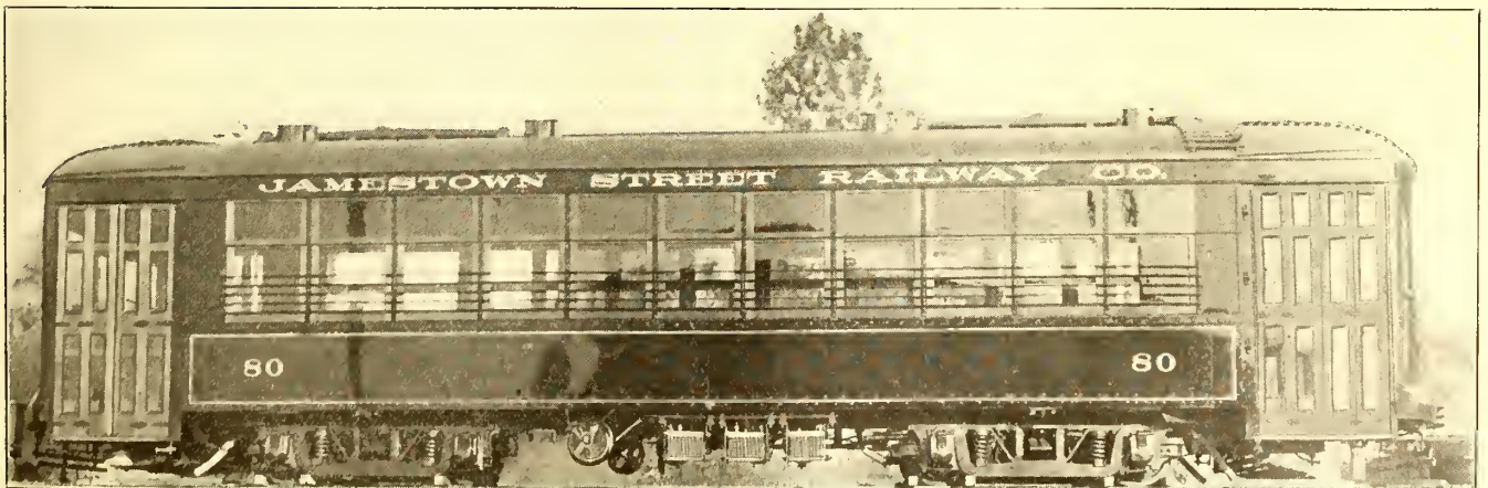
JAMESTOWN STREET RAILWAY'S NEW DOUBLE-TRUCK, FLUSH PLATFORM CAR FOR CITY SERVICE
