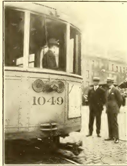
REAR OF A CAR OF THE CLEVELAND RAILWAY EQUIPPED WITH INDICATING TAIL LIGHTS
