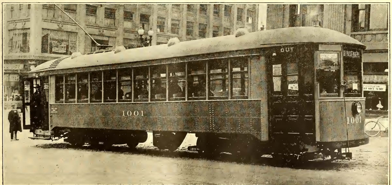
LIGHT-WEIGHT SEMI-STEEL CAR BUILT IN OMAHA SHOPS
