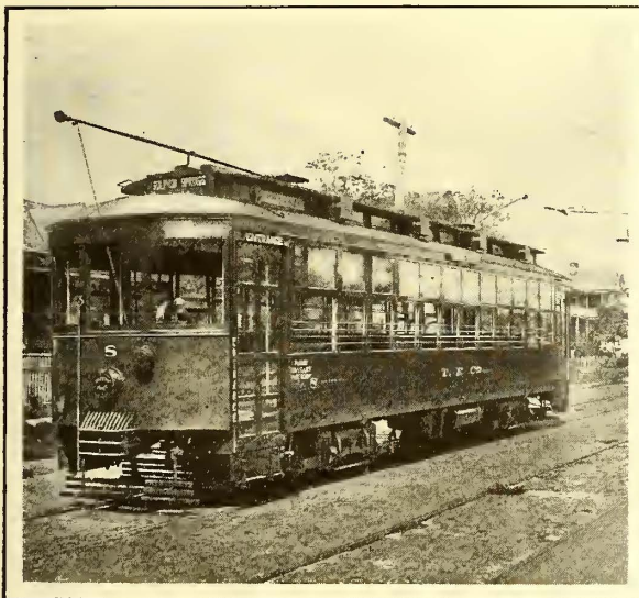
Large Car Rebuilt for Operation with Safety Devices Combination
