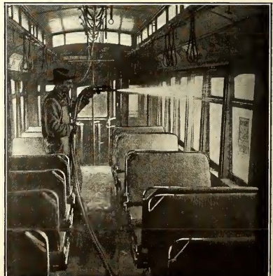
AT LEFT, WASHING CARS ON THE OUTSIDE WITH SPECIAL SPRINKLING SYSTEM AT EAST ST. LOUIS. AT RIGHT, METHOD OF CLEANING CAR INTERIORS
